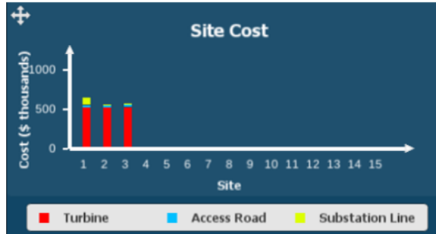
Figure 18: Site Cost graph from viewscreen. For each turbine, the red bars indicate the cost of the turbine, the blue bars the cost of the access roads, and the yellow bars the cost of the substation lines.
